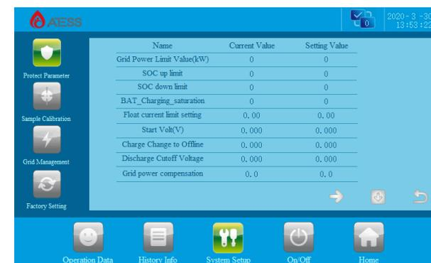
**Grid power limit value:** the upper limit of power that can be taken from grid, which only takes effect under peak shaving mode, and the default maximum setting is twice of the rated power(maximum for HPS150 is 240).
