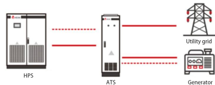
3. There are three circuit breakers in ATS. The middle circuit breaker is connected to the power grid switch (AC input) of HPS. The other two are grid switch (grid) and generator (Gen) switch. Pay attention to the printing on cabinet. It is not allowed to connect incorrectly, neither is it for the three phase sequence, otherwise the system cannot operate normally.
