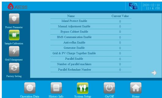
**Islanding protection enable:** it is a protection to prevent the inverter from not correctly switching into off grid mode in case of grid abnormality. Enter 0-9,0 means disable; 1-9 means level, suggested not to set too high.
