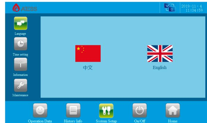
**Time settings:** system time setting (if the date and time displayed on LCD is not inconsistent with the actual date and time, they can be modified here).
