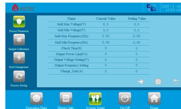
**Grid Max. voltage:** If it exceeds Max. power grid voltage, it will switch to off grid mode. The default setting is 110% of rated voltage.
