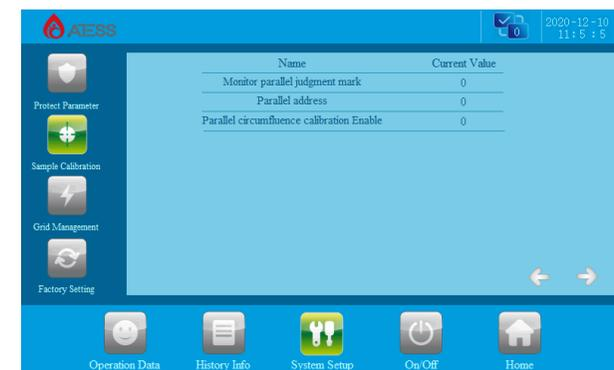
**Monitoring parallel judgment mark:** when the system is parallel system with Shinemaster monitoring, the same value will be set for the energy storage controller of the same system, and the parallel system data will be automatically counted on the monitoring page, otherwise the single machine data will be recorded. When set to 1 means the function is disabled.
