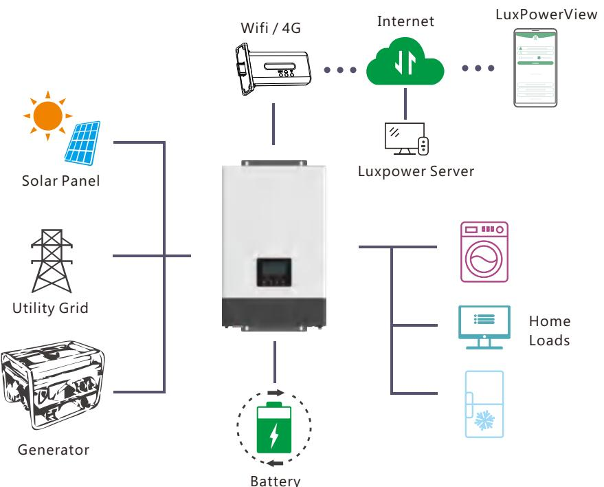
SONAR series is a multifunctional, high frequency pure sine wave ECO Hybrid inverter solar inverter, features:
