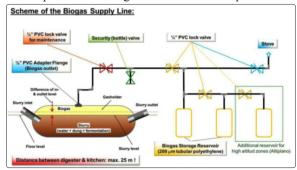
**Source:** Installation manual for Low-Cost Polyethylene Tube Digesters
